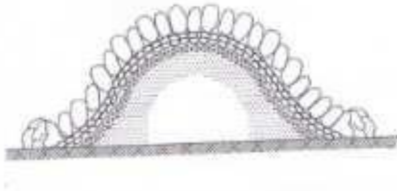
Fig. 14.2. A Rubble mound breakwater
