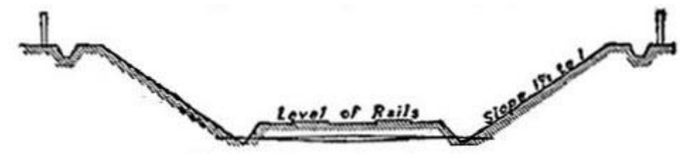
Typical Section of Railway in Cutting.
