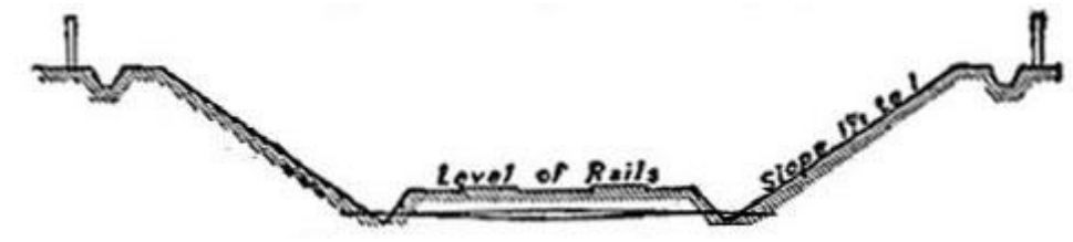
Typical Section of Railway in Cutting.
