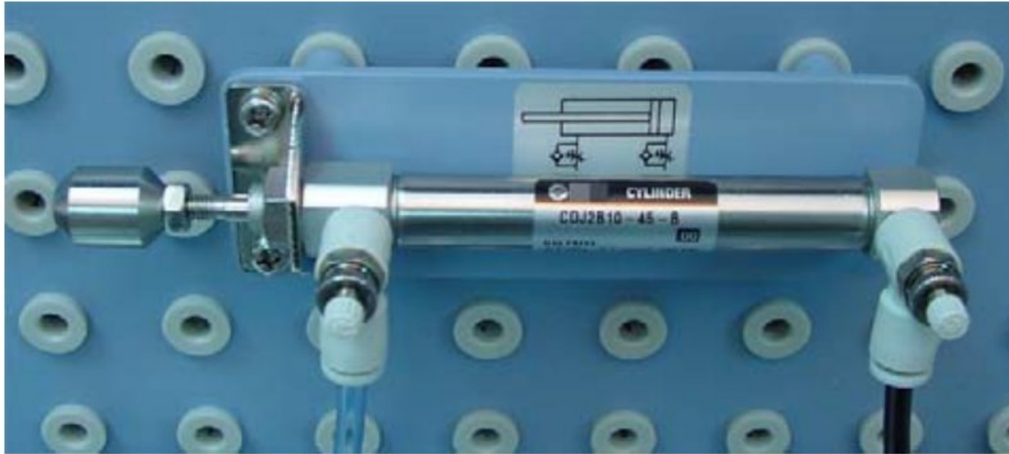
a) Double acting cylinder
